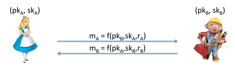
$$KDF(pk_B,sk_A,r_{A,m_B}) = k_{AB} = KDF(pk_A,sk_B,r_{B,m_A})$$
