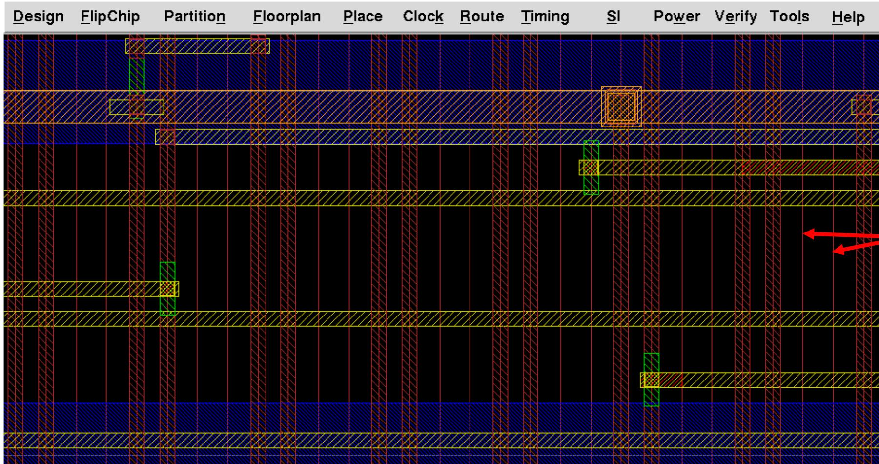
Routing forbidden: tracks obtrusted = shield
