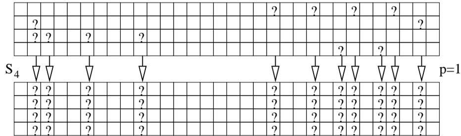
We checked all the various outputs of this  $S_4$  and found that all the possible output differences do not affect the linear approximation used in the attack. The empty arrow means that this holds with probability 1.
