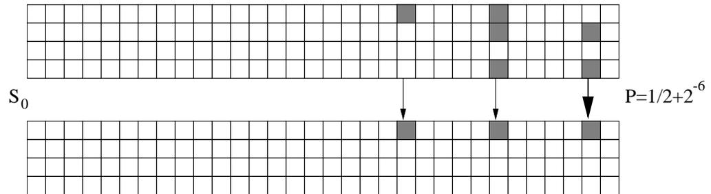
After the linear transformation, and the application of  $S_1$  we get the following linear approximation with bias of  $2^{-7}$ :
