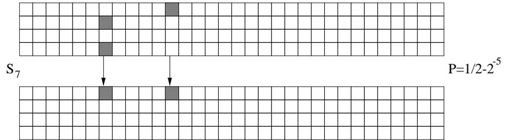
After the linear transformation, and the application of  $S_0$  we get the following linear approximation with bias of  $2^{-6}$ :
