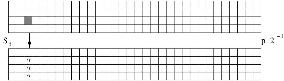
Where the '?' means that we do not care what the value of the difference is, and the bold and thick arrow means that this happens with probability  $1/2$ . After the linear transformation, we get the following truncated differential in the input to  $S_4$ :
