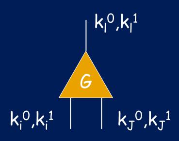
$k_i^0 = 0$  on wire i  $k_i^1 = 1$  on wire i
