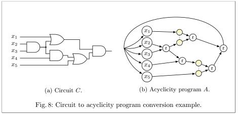
evaluates to false. If top is AND, then at least one of the subcircuits is false and the paths in it cannot all be covered. If top is OR, then both subcircuits are false, so at least one of them cannot be covered regardless of the choice of  $y_i$  and  $z_i$ .
