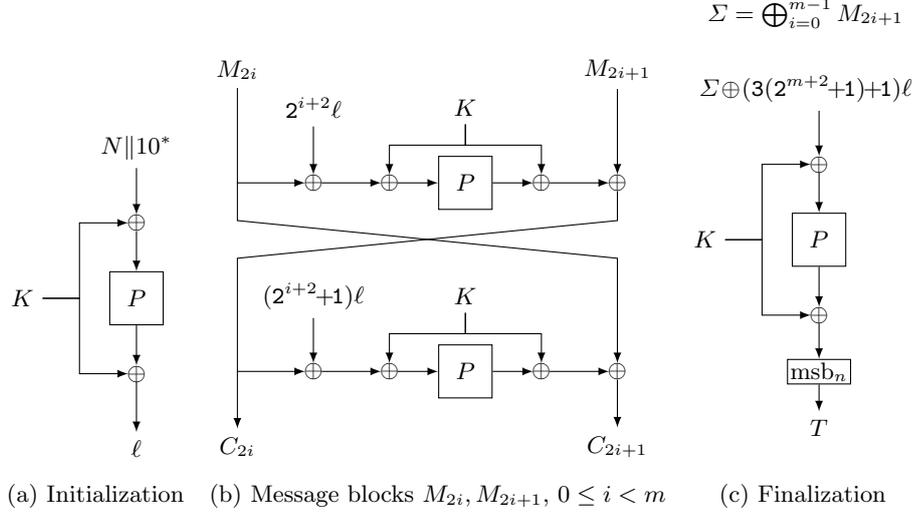
Fig. 1: Encrypting  $2m$  message blocks  $M_j$  with Prøst-OTR- $n$  under key  $K$  and nonce  $N$ . All values are  $2n$  bits, with  $n \in \{128, 256\}$ , except the  $n$ -bit tag  $T$ .
