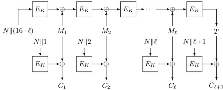
Fig. 4: CCM encryption.
