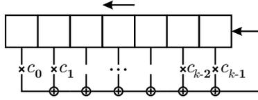
**Fig. 1.** An LFSR corresponding to the companion matrix  $C$  of polynomial  $g(X) = X^k + c_{k-1}X^{k-1} + \dots + c_0$ . Clocking it  $k$  times is equivalent to applying  $C^k$  to its internal state.
