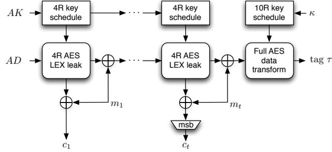
**Fig. 3.** Processing message and finalization in ALE.
