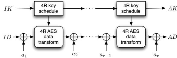
**Fig. 2.** Processing associated data in ALE.
