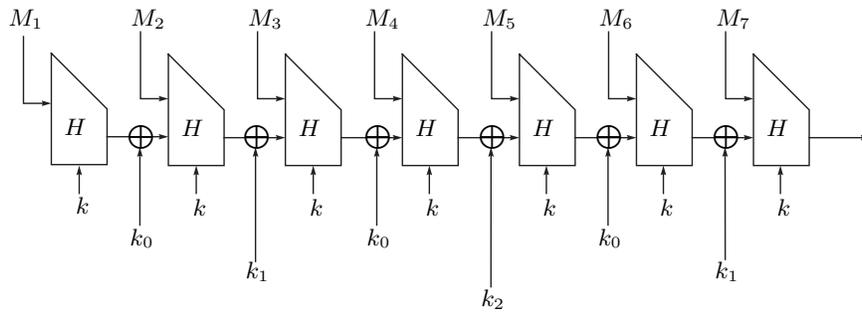
**Fig. 1.** Extenders for TCR hashes: linear, basic tree, and Shoup constructions.
