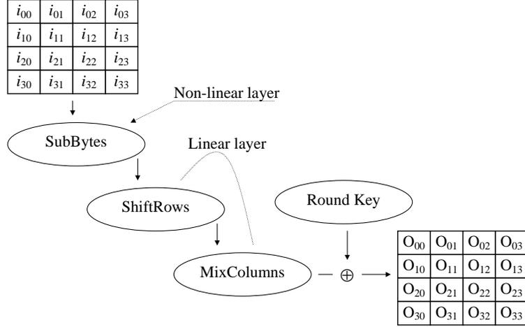
**Fig. 1.** Basic structure of the *AES* algorithm
