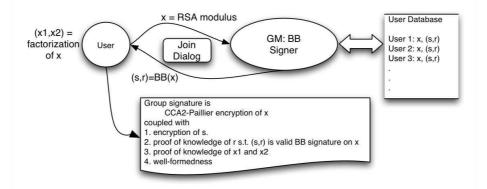
Fig. 1. Overview of our general group signature design. The BB signature can be substituted by potentially other signatures that are suitable for algebraic encryption with efficient validity proof.
