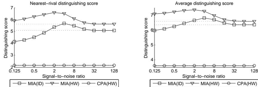
**Fig. 3:** The effect of Gaussian noise on HW and ID attacks against HW leakage of the first DES S-Box.
