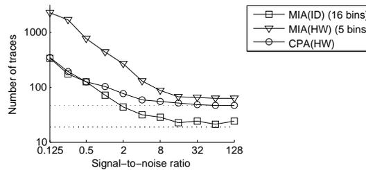
**Fig. 6:** Average number of traces required for key recovery in simulated practical attacks against Hamming-distance leakage (with a reference state of  $0100_{(2)}$ ), for varying levels of Gaussian noise.
