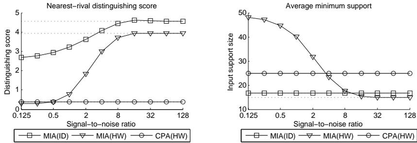
**Fig. 5:** Nearest-rival distinguishability and required support size of theoretic attacks against Hamming distance leakage (with a reference state of  $0100_{(2)}$ ) for varying levels of Gaussian noise.
