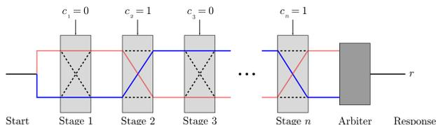
**Fig. 1.** Schematic of an  $n$ -bit Arbiter PUF.
