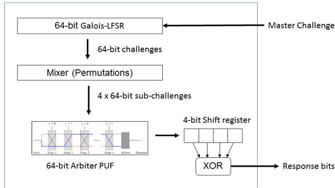
**Fig. 3.** Internal structure of the PUF tag. A 64-bit Galois LFSR is used to generate challenges from a master challenge. Each challenge is fed into the mixer function which generates four subchallenges by permuting the input challenge. These four subchallenges are successively fed into the 64-stage Arbiter PUF. The four responses of the Arbiter PUF are then XORed to provide a response bit that is sent to the reader.
