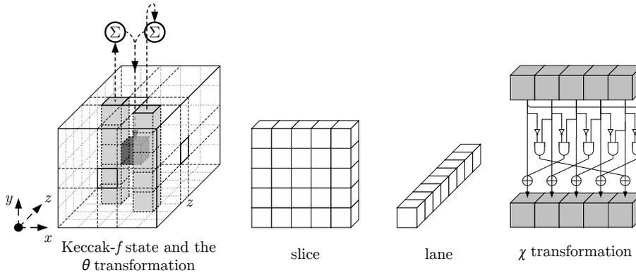
**Fig. 1:** Parts of the KECCAK- $f$  state [7] including  $\theta$  transformation (left) and  $\chi$  transformation (right)<sup>2</sup>
