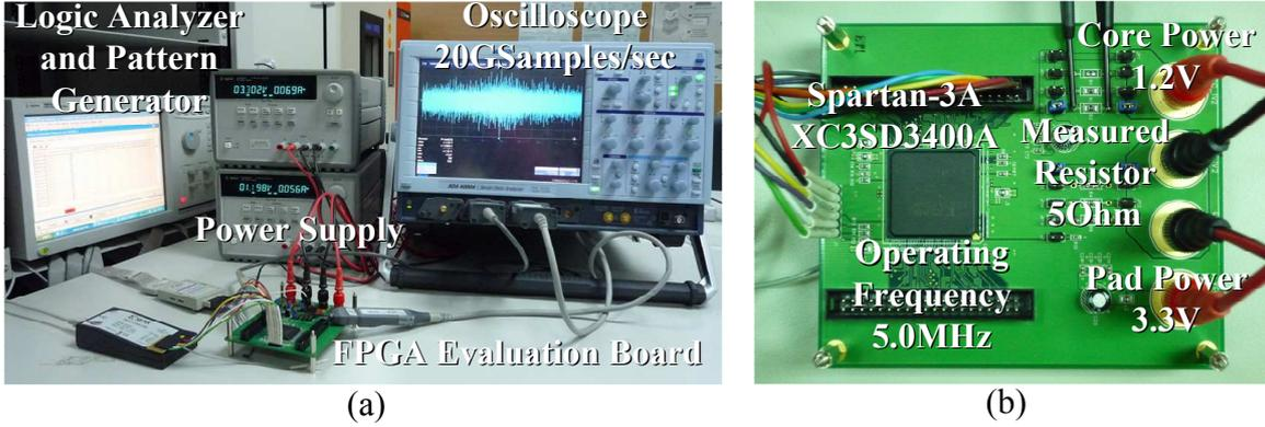
**Fig. 7.** (a) Environment of power measurement. (b) Current running through the DF-ECC processor recorded by measuring the voltage drop via a resistor in series with the board power pin and FPGA power pin.
