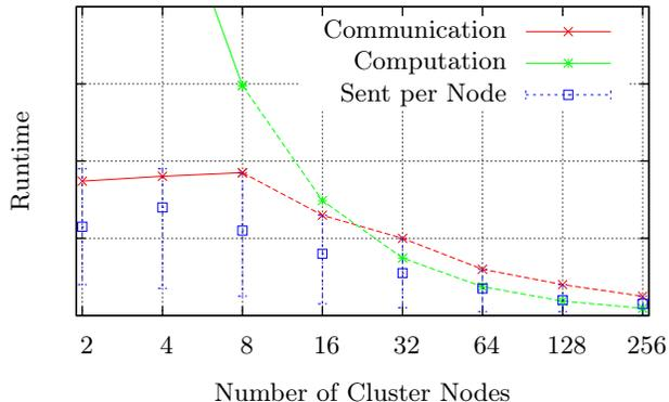
**Fig. 4.** Estimation of computation time vs. communication time on a cluster system. The numbers for 2, 4, and 8 nodes are measurements, the numbers for larger cluster sizes are estimations. The amount of data sent per node varies; we show the maximum, minimum, and average.
