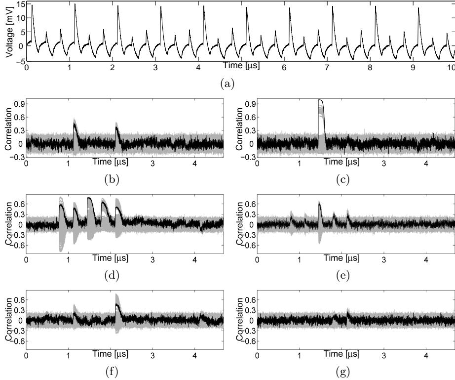
**Fig. 6.** **BRAM** version, (a) sample power trace, collision attack results by register update model, (left) first-order (right) second-order: (b) and (c) **Conventional**, (d) and (e) **First CT-RSA**, (f) and (g) **Second CT-RSA** profiles, each using 1 000 000 traces
