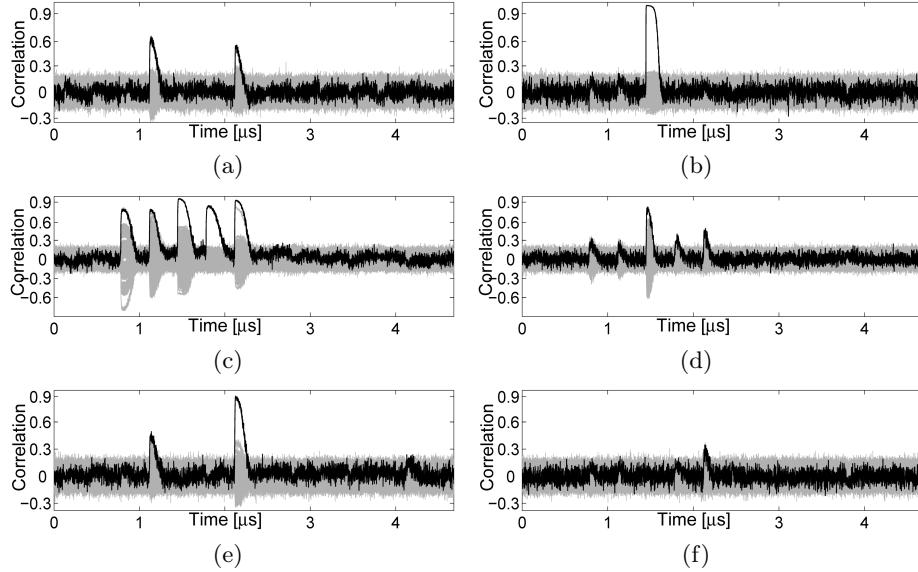
**Fig. 7.** BRAM version, collision attack results by S-box input model, (left) first-order (right) second-order: (a) and (b) **Conventional**, (c) and (d) **First CT-RSA**, (e) and (f) **Second CT-RSA** profiles, each using 1 000 000 traces
