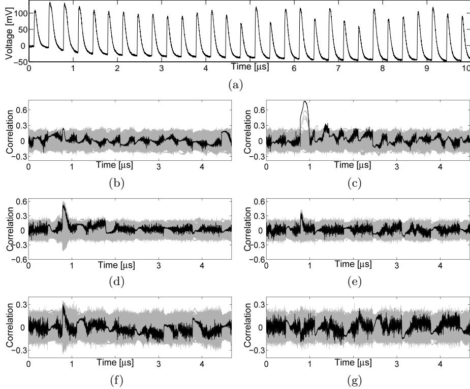
**Fig. 4.** **LUT** version, (a) sample power trace, collision attack results by register update model, (left) first-order (right) second-order: (b) and (c) **Conventional**, (d) and (e) **First CT-RSA**, (f) and (g) **Second CT-RSA** profiles, each using 1 000 000 traces
