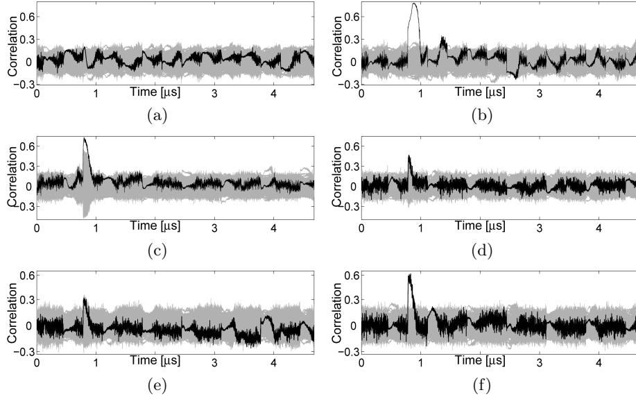
**Fig. 5.** LUT version, collision attack results by S-box input model, (left) first-order (right) second-order: (a) and (b) **Conventional**, (c) and (d) **First CT-RSA**, (e) and (f) **Second CT-RSA** profiles, each using 1 000 000 traces
