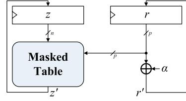
**Fig. 2.** CT-RSA masking architecture [10]
