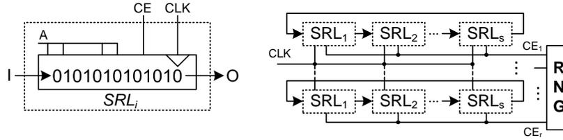
**Fig. 1.** Noise generation based on shift-register LUT (SRL)
