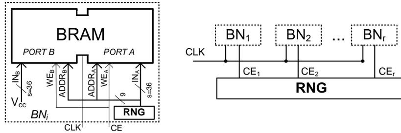
Fig. 2. Noise generator based on memory write collisions
