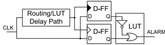
Fig. 5. Circuit to detect external clock manipulations
