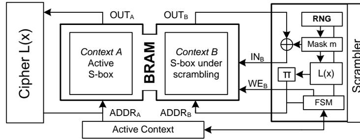
Fig. 6. Construction scrambling S-box entries with random masks
