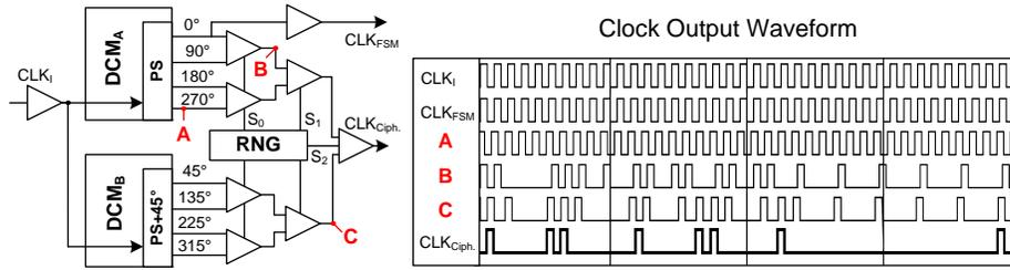
Fig. 4. Clock randomization using DCMs and a tree of clock buffers
