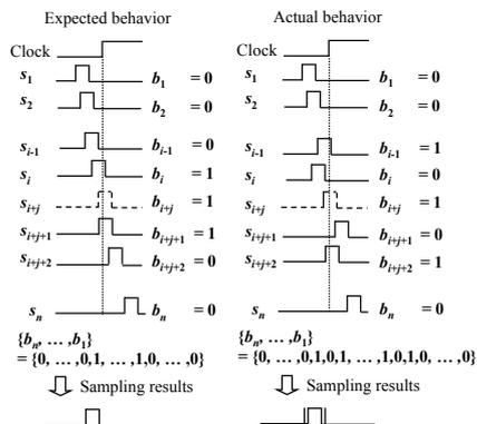
Fig. 4. Error in glitch acquisition
