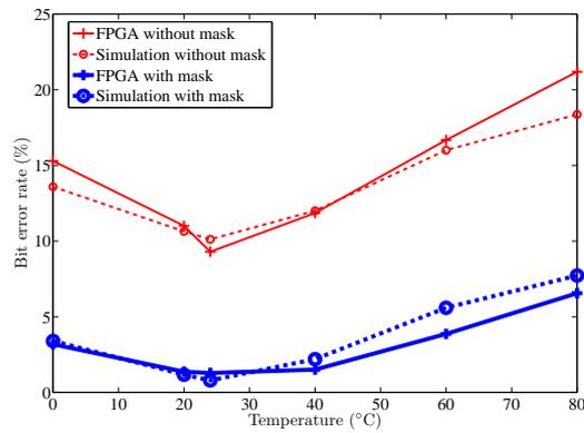
Fig. 17. Change of error rate accompanying temperature change
