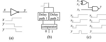
**Fig. 2.** Circuit behaviors for different delay values
