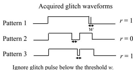
**Fig. 8.** Conversion from glitch waveform to response with filtering
