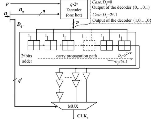
Fig. 11. Variable delay circuit
