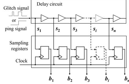
**Fig. 3.** Sampling circuit
