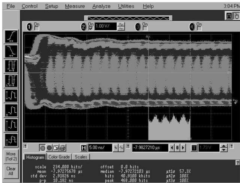
Fig. 8. Histogram of phase distribution in Meta-RO5st digital TRNG. The phase distribution occupies the whole period of the Meta-RO oscillations, significantly increasing the entropy
