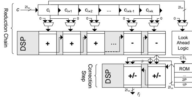
**Fig. 5.** Modular reduction for NIST-P-224 and P-256 using DSP blocks
