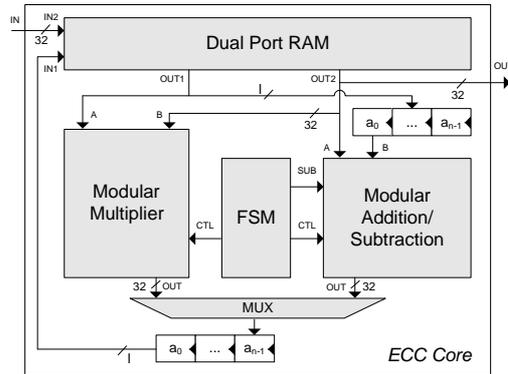
**Fig. 6.** Schematic overview of a single ECC core
