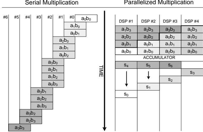
**Fig. 3.** Parallelizing multiplication for efficient DSP-based computation
