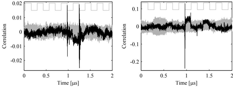
**Fig. 3.** Results of the DPA attacks on the DRP core (left, 300000 samples) and the MDPL core (right, 5000 samples): internal MOV operation in the IRAM, correlation trace for correct power hypothesis is plotted in black.
