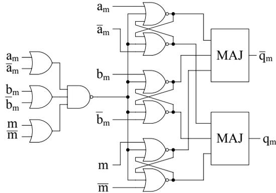
**Fig. 7.** An iMDPL-AND cell. The original MDPL-AND cell only consists of the two Majority cells MAJ.
