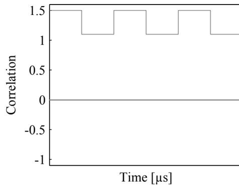
**Fig. 9.** Result of the DPA attack on the iMDPL core: transition count based on logic simulation of internal MOV operation in the IRAM, 256 samples, correlation trace for correct power hypothesis is plotted in black.
