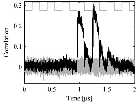
**Fig. 2.** Result of the DPA attack on the CMOS core: internal MOV operation in the IRAM, 5000 samples, correlation trace for correct power hypothesis is plotted in black.
