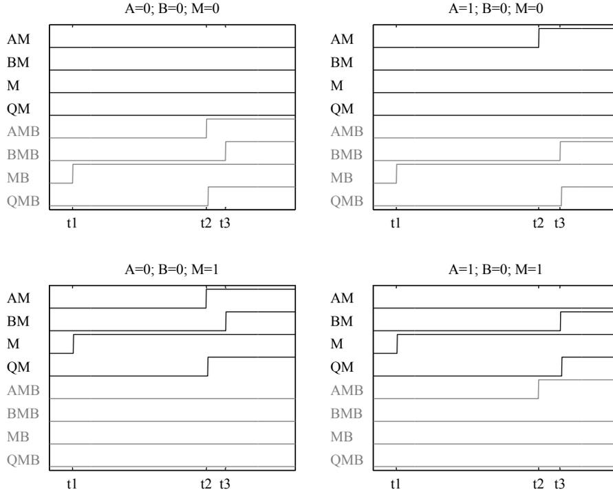
**Fig. 5.** Signals for the MDPL-AND Majority cells for which early propagation occurs (transistor-level simulation, black: signals of first MAJ cell, gray: signals of second MAJ cell). Signal  $A$  depends on the moved value. Signal  $B$  is constantly 0.
