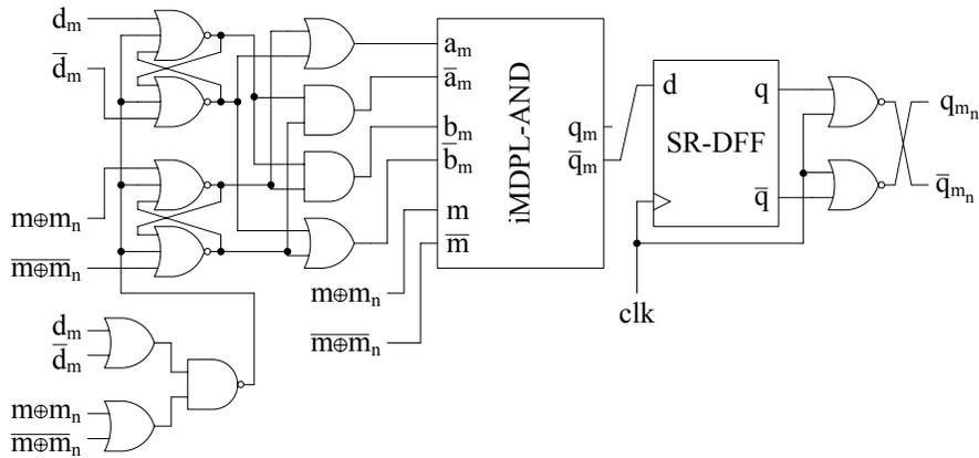
**Fig. 8.** An iMDPL-DFF. The original MDPL-DFF does not have the two input latches and the EPDU.
