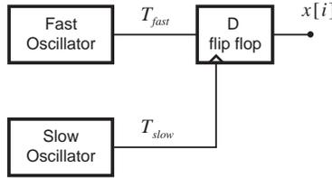
**Fig. 3.** Oscillator-based RBG.
