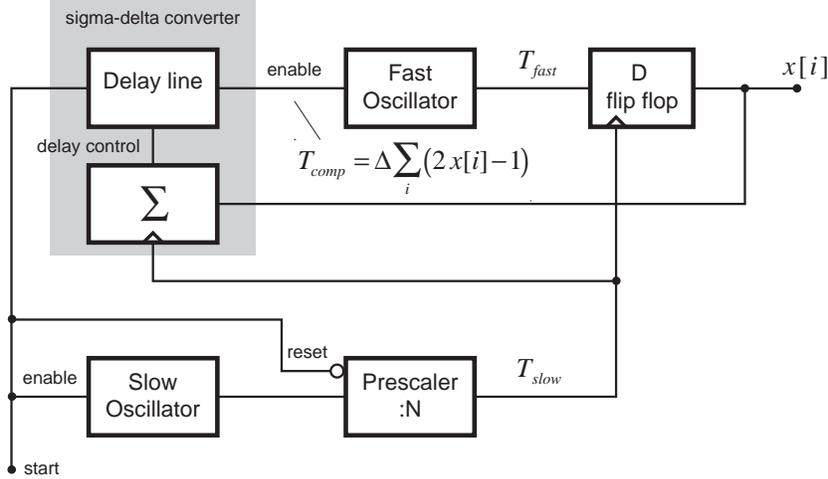
Fig. 5. The RBG proposed in this work.
