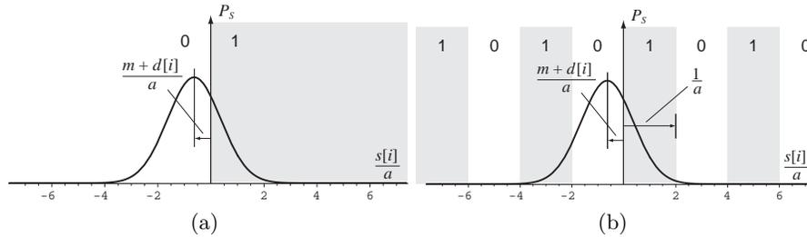
**Fig. 1.** Source quantization modes: (a) sign-mode ( $x[i] = \text{sign}(s)$ ), (b) mod 2-mode ( $x[i] = \lfloor s \rfloor \text{mod } 2$ ).
