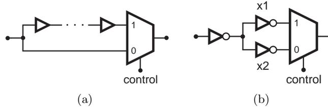
**Fig. 9.** Implementation of the coarse (a) and fine (b) differential delay elements. The fine delay cell exploits the differential delay between two inverters having different drive strength ( $x1$  and  $x2$ ). Since the inverters are driven in parallel, inputs signals are aligned while, on the output, the stronger inverter ( $x2$ ) switches faster.
