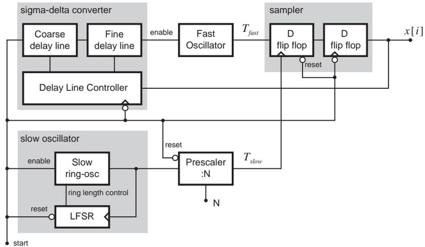
**Fig. 7.** Detailed block scheme for the proposed RBG.
