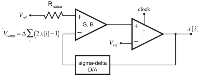
**Fig. 2.** Amplification-based RBG.
