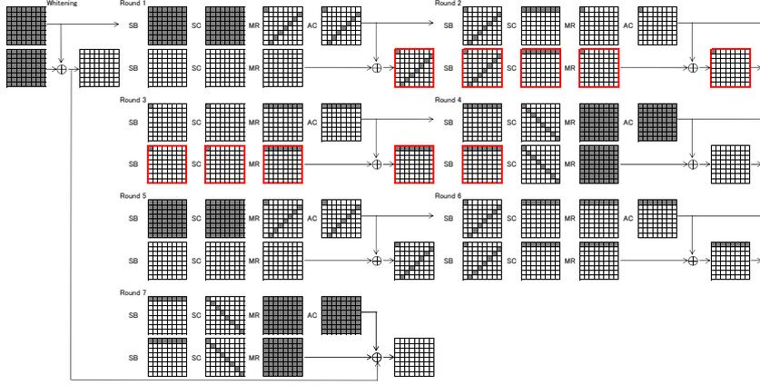
**Fig. 4.** Differential path for 7R attack. Grey bytes are active bytes. The inbound phase for the data processing part is stressed by red squares.
