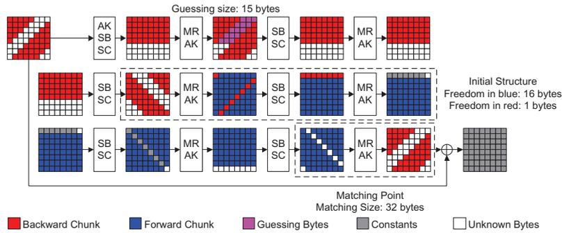
**Fig. 6.** Chunk separation  $(b, r, w, g) = (7, 5, 1, 5)$  for the memoryless second preimage attack on 6-round hash function
