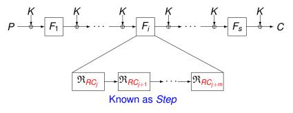
Block ciphers like LED-64, PRINCE<sub>core</sub>, Zorro and PRINTcipher.
