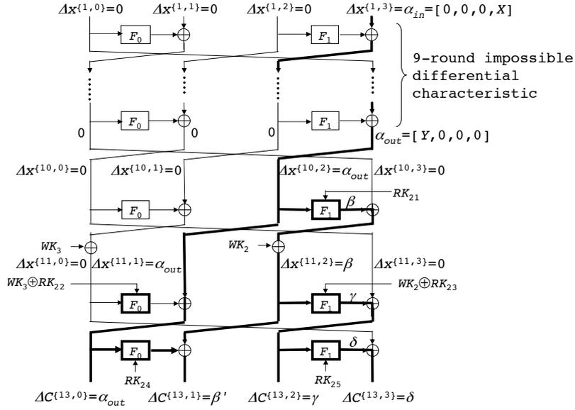
Fig. 6. Impossible differential attack on 13-round CLEFIA
