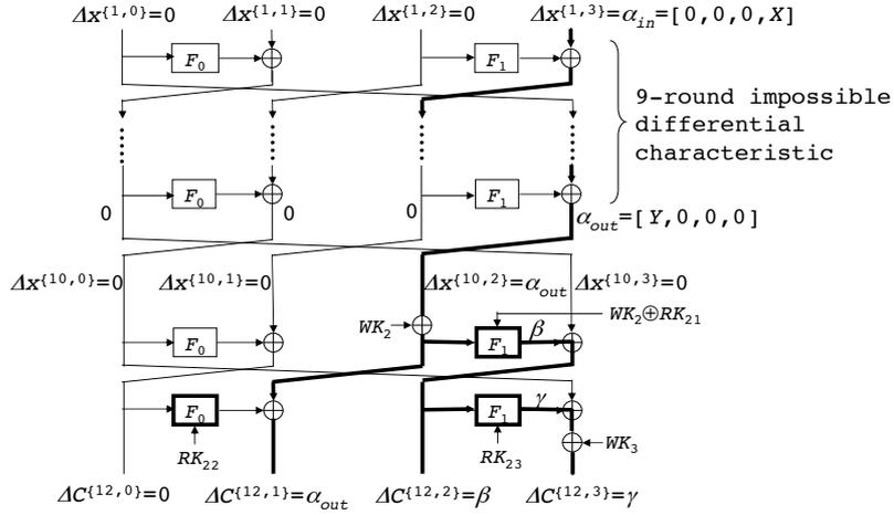
Fig. 4. Impossible differential attack on 11-round CLEFIA
