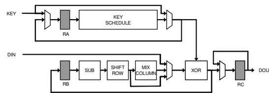
Fig. 2. Architecture of AES core
