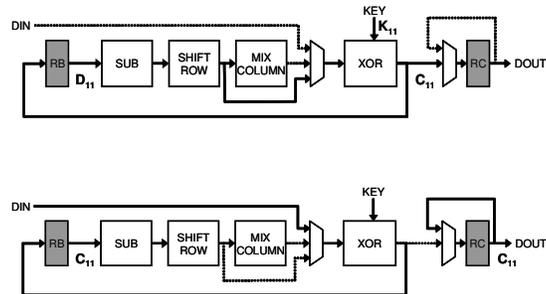
Fig. 5. AES core: round 11 (top); and round 11 + 1 (bottom)
