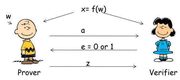
Has error probability  $\frac{1}{2}$ . Can be amplified to 2<sup>-n</sup> by iterating n times. Means proof has size O(kn) bits, k size of problem instance.
