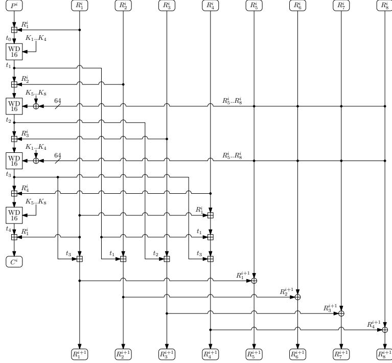
**Fig. 3.** Encryption of plaintext word  $P^i$  to ciphertext word  $C^i$  and update of state  $R$ . The “temporary” variables  $t_0 \dots t_4$  are used in the description of the attack.
