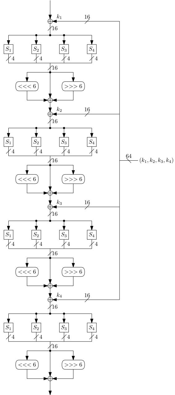
**Fig. 1.** The “WD16” mixing function is a 16-bit substitution-permutation network with four rounds and a 64-bit subkey  $(k_1, k_2, k_3, k_4)$ . It is used in both initialization and encryption phases.
