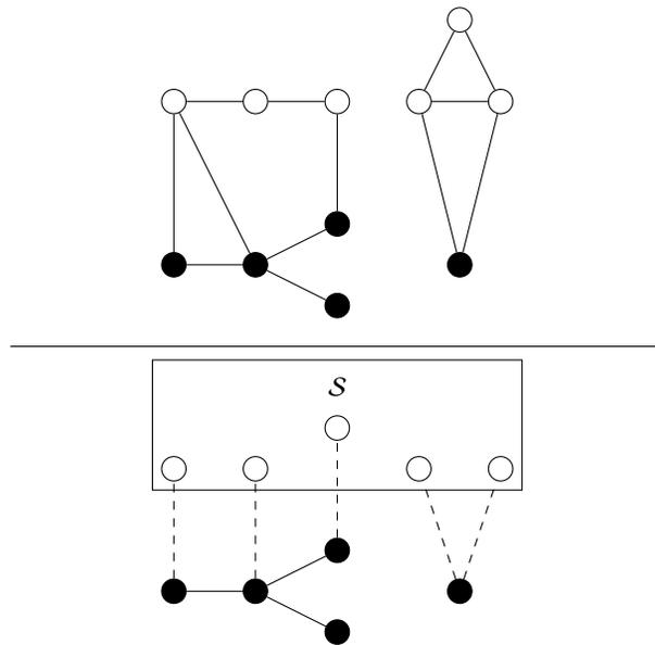
Fig. 3.1: An example of how the simulator works. The top shows how the graph normally looks. The bottom shows the graph topology that the simulator generates. Black nodes are nodes in  $Q$ . Notice that the simulator doesn't require knowing if nodes in  $Q$  have a common neighbor — neighbors can identify themselves with pseudonyms or edge-labels.
