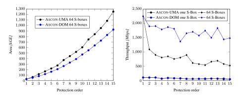
**Fig. 10.** UMA versus DOM area requirements for different protection orders and 64 parallel S-boxes (left) and throughput comparison in the right figure
