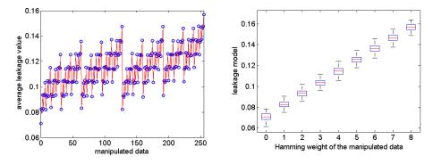
Fig. 1: PIC leakage model: average values (left) and grouped by HWs (right).
