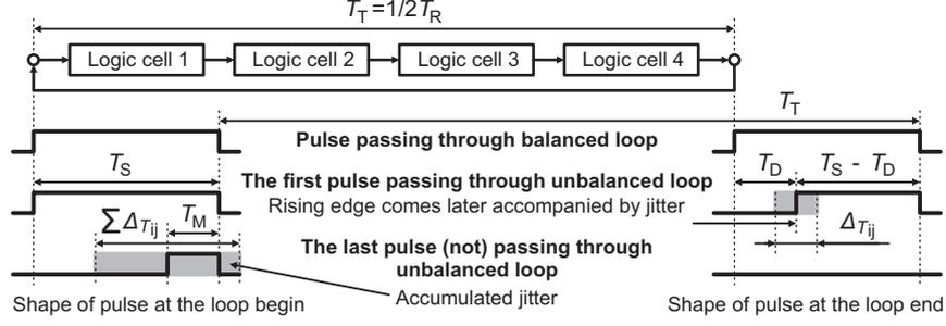
**Fig. 4.** Graphical representation of the mathematical model, where the instability of the pulse shortening during circulation around TERO is a key issue. Therefore the pulse will disappear after several oscillations.
