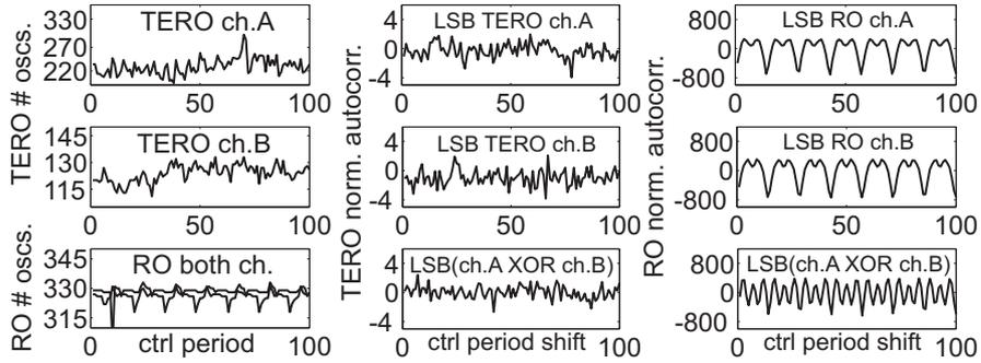
**Fig. 10.** TERO and RO mode comparison in hardware. Channels A and B are synthesized in the closest CLBs. Left column shows number of oscillations for both channels of TERO and RO in 100 consecutive *ctrl* periods. Normalized autocorrelation of TERO channels A and B and their XOR combination for 1–100 *ctrl* periods shift is given in the middle column. The same results, but for RO mode is depicted in right column.
