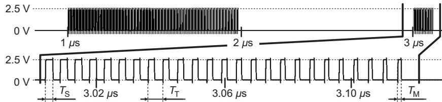
**Fig. 3.** LT Spice simulation of the TERO. TERO starts to oscillate at the rising (1  $\mu$ s) or falling (3  $\mu$ s) edge of the *ctrl* signal having a 4  $\mu$ s period. Zoomed region shows that excited pulse disappears due to its shortening each loop crossing.  $T_T$  stands for the mean value of the oscillation period,  $T_S$  and  $T_D$  denote time durations of logic '1' level when oscillation behavior raises and disappears respectively.
