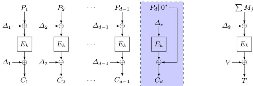
**Fig. 3.** Encryption in OCB.
