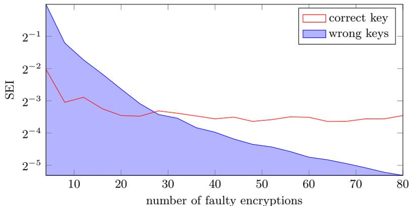
**Fig. 7.** SEI values for correct key ( $SEI_c$ ) plotted against best SEI for a wrong key ( $\max(SEI_w)$ ) for increasing number of faulty encryptions. Setup: AES software implementation, single clock glitch.
